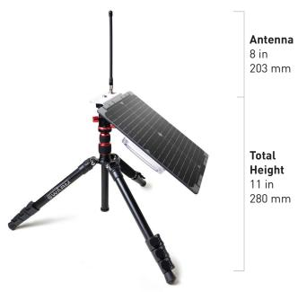
The Swarm Eval Kit transmits and receives data to and from Swarm's satellite network to provide connectivity anywhere on Earth. The Eval Kit is designed to provide the developer with an easy-to-use platform, with the included FeatherS2 - ESP32 board + OLED, a USB-C port, and I2C port for sensors. FeatherWing add-on modules can provide a suite of additional capabilities.
