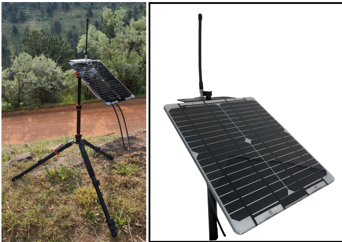
Figure 10: Example \frac{1}{4} -wave antenna with a (Swarm) 9W solar panel serving as the required 30 x 30 cm ground plane off to one side. Tested extensively in the field and works well.
